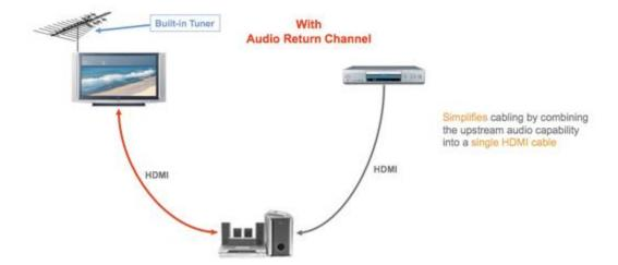
Unlike previous versions of the sound output when it was necessary to use external speakers. Reverse channel will allow to take such a signal from the air and listen to the sound using HDMI to the connected speakers.
